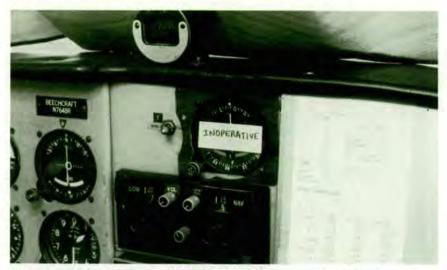
Although two VOR indicators make it easier to navigate around the ARSA, the good one on the left meets the pilot's minimum standard for a safe VFR flight.
