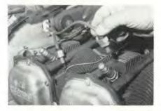
Due to the different polarity each plug receives from the magneto system, spark plugs on the bottom should be periodically rotated with those on top.
