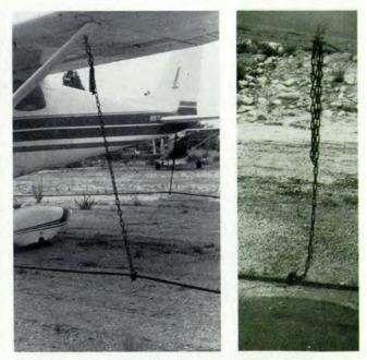
Chains are often used in place of rope. Fastened too tightly, like the chain to the left, chains can cause immediate overstress in a gust.
