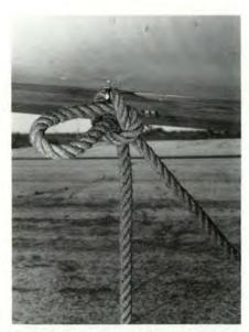
Here's the wing of a \$100,000 airplane "secured" with a \$20 rope and a 10-cent slipknot.
