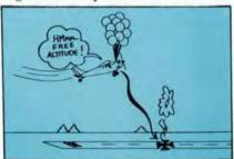
cipient rising early, it can be dealt with by lowering the nose slightly. However, a ballooning aircraft can leap 20 to 30 feet with little warning. In this case, avoid the temptation to lower the nose to put the aircraft on the runway. Instead, maintain the pitch, and add enough power to allow the aircraft to settle gently on the runway. Or, GO AROUND.
